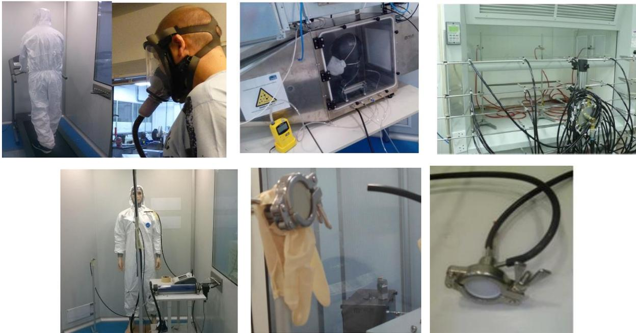
Figure 3. Samples of some experimental set ups for RMMs testing: masks (upper left), LEVs (upper right), suits (down left) and gloves (down right).
